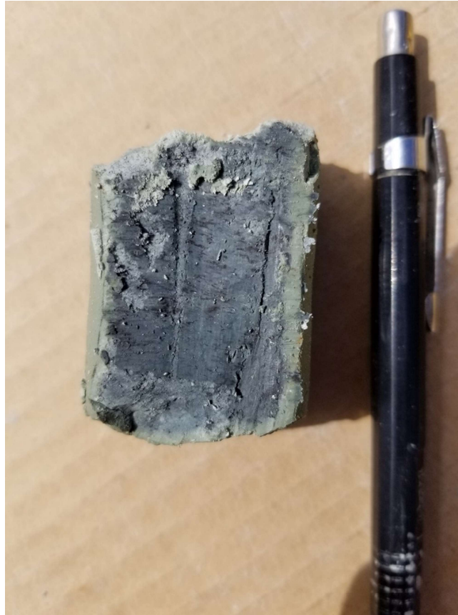
Figure 7-7: Split reduce core after about one week's exposure to air
